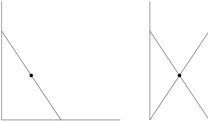
Another situation which exhibits the same phenomenon is that of a collapsible ironing board, that has a pair of legs crossed at their midpoints. The end of one leg is fixed to the end of the ironing board; the end of the other is free to travel along the ironing board. What is the path traced out by the crossing point when the ironing board is opened.
