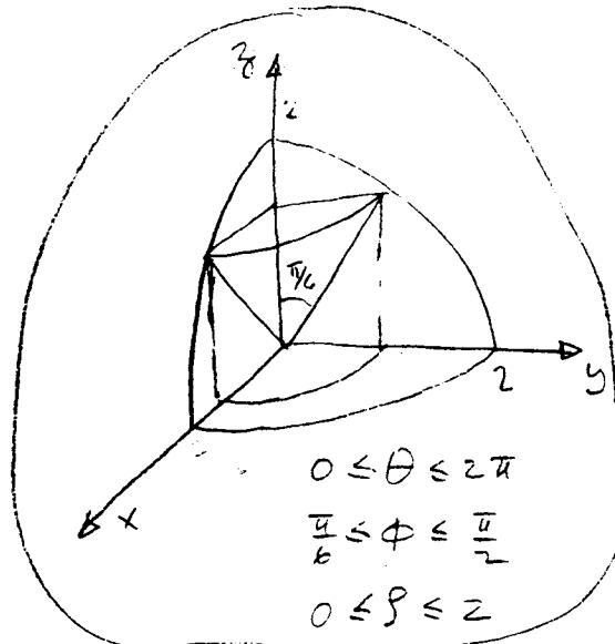
$$M_{xy} = \int_0^{2\pi} \int_{\frac{\pi}{6}}^{\frac{\pi}{2}} \int_0^2 \rho^3 \sin \phi \cos \phi d\rho d\phi d\theta$$
